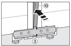
■ Position the long stainless steel trim ① in the gap, making sure that it is located above bracket ③.
